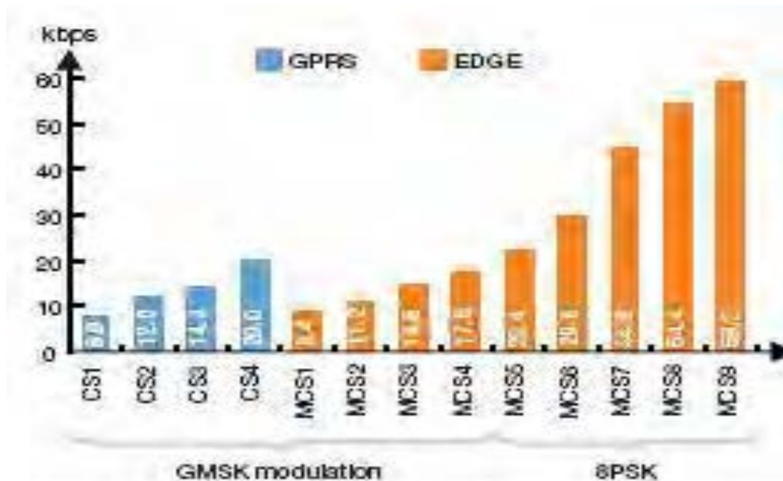
Figure 4. Coding schemes for GPRS and EGPRS (user data rate). (Key: 8PSK, 8-phase shift keying; CS, Coding scheme; EGPRS, Enhanced GPRS; GMSK, Gaussian minimum shift keying; MCS, Modulation coding scheme)
